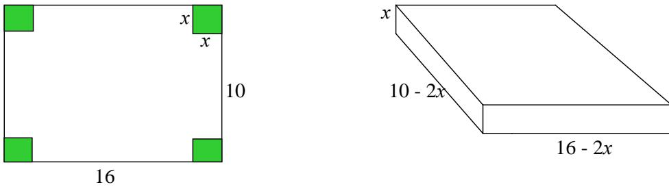
$$V_{\text{box}} = x(10 - 2x)(16 - 2x), \quad x = ? \text{ for max } V$$
