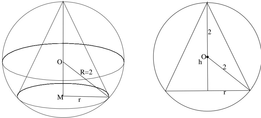
$$V_{\text{cone}} = \frac{\pi}{3} r^2 h \quad OM = h - 2 \Rightarrow 4 = r^2 + (h - 2)^2$$
